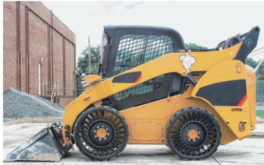
Michelin's airless tire, called the Tweel, shown on a front end loader. (COURTESY OF MICHELIN NORTH AMERICA)
